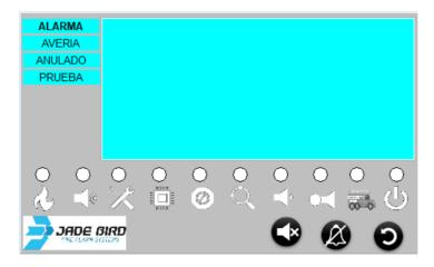
Reset: This is the key that allows the control panel to be reset and cancels all alarm incidents,
