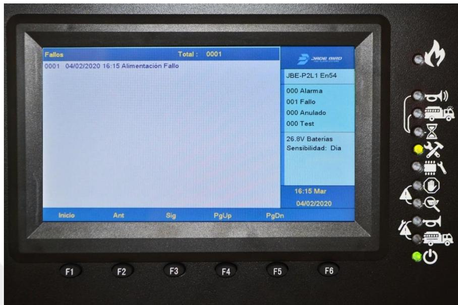
Figure 21: Fault Screen
