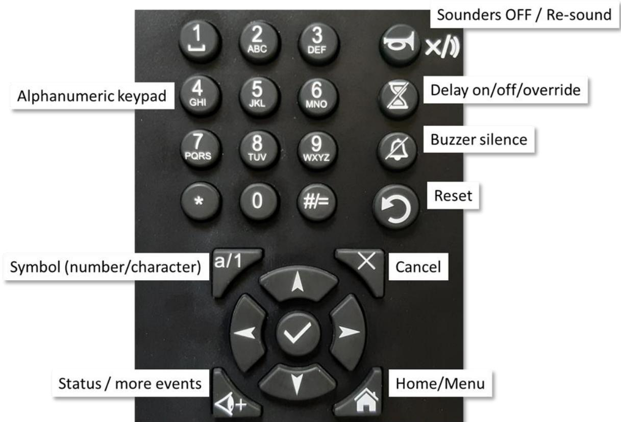
Figure 12: Control keys and alphanumeric keyboard
