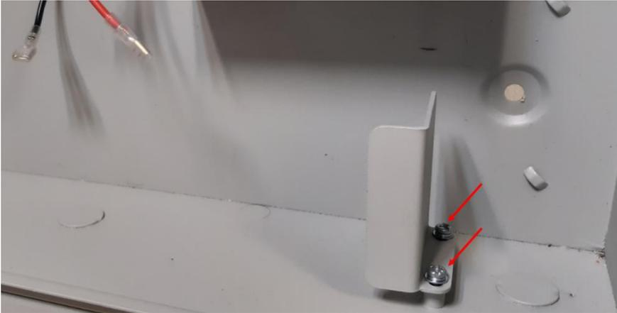
Figure 7: Battery Holder Brackets
