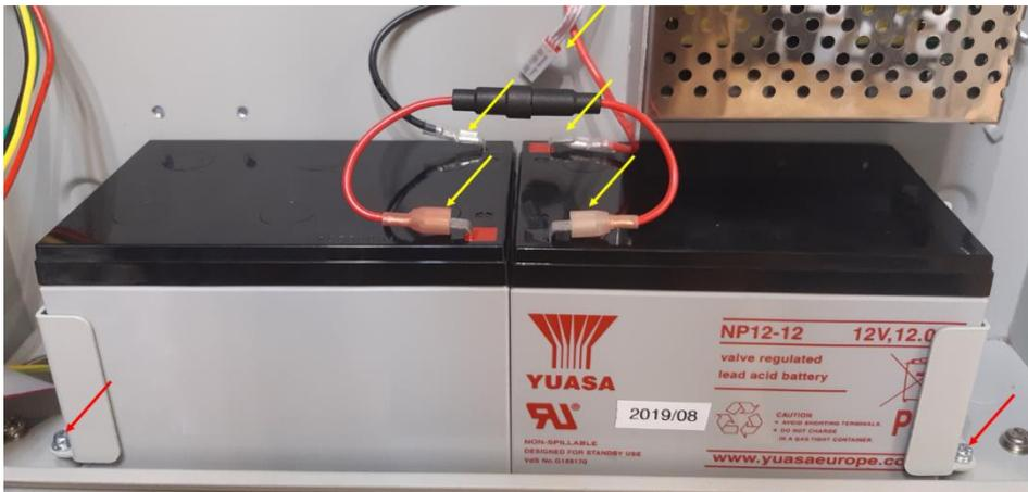
Figure 8: Battery Connection Locations for 7 & 12 Ah
